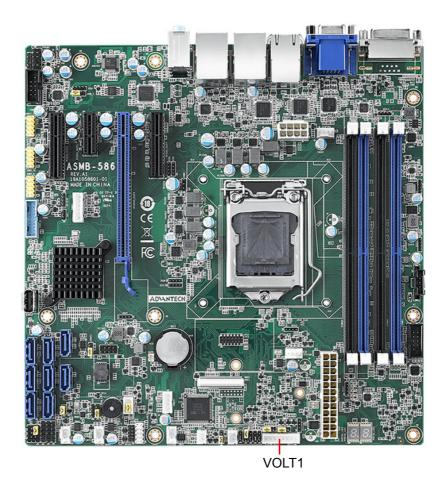
VOLT1 connects to the alarm board of Advantech chassis. This alarm board monitors the input voltage of +12V, +5V, +5Vsb, -5V +3.3V and -12V, and give warnings if a power supply fails.
