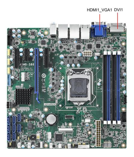
The ASMB-586 is equipped with VGA, DVI-D and HDMI connectors for triple display output. However, results may differ because of OS support limitations.
