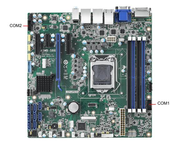
The ASMB-586 offers two serial ports onboard, COM1 and COM2 (one can be connected to rear panel via the dedicated COM cable kit in the accessory box) for the use in a serial mouse, printer or communications network, etc. The IRQ and address ranges for those ports are fixed. However, if you want to disable the port or change these parameters later, you can do this in the system BIOS setup. Different devices implement the RS-232 standards in different ways.
