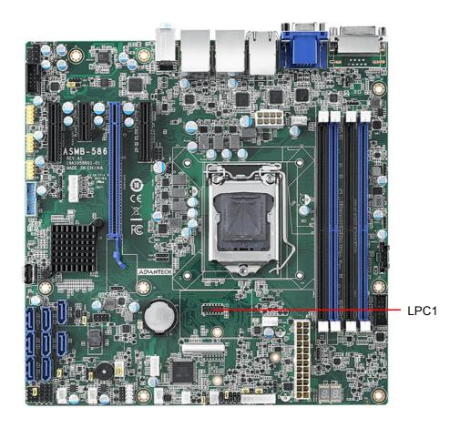
LPC connector on ASMB-586 is reserved for Advantech TPM and COM RS-232/422/485 modules.
