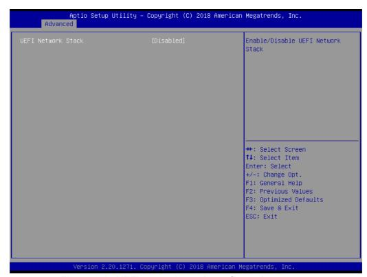
Figure 3.19 UEFI network stack configuration screen
